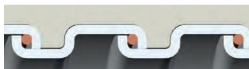
Square-Locked Design with integral bonding wire 3/8" through 1-1/4"
