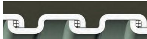
Square-Locked Design with cord packing 3/8" through 1-1/4"
