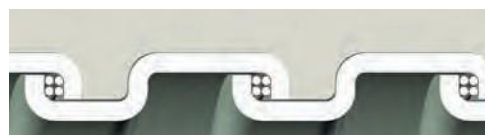
Square-Locked Design with cord packing 3/8" through 1-1/4"
