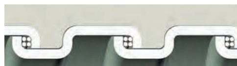
Square-Locked Design with cord packing 3/8" through 1-1/4"
