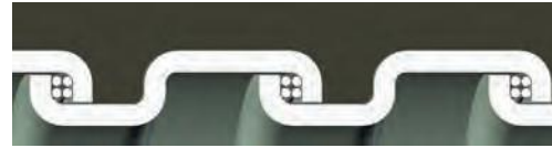
Square-Locked Design with cord packing 3/8" through 1-1/4"
