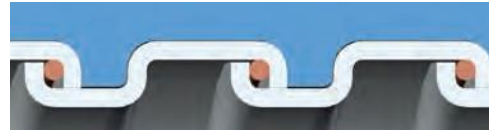
Square-Locked Design with integral bonding wire 1/2" through 1-1/4"
