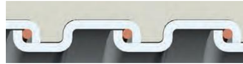
Square-Locked Design with integral bonding wire 3/8" through 1-1/4"
