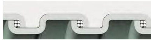
Square-Locked Design with integral bonding wire 3/8" through 1-1/4"
