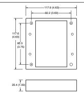
Extension WE2 – Dimensions in Millimeters (Inches) Extensions and Extension Adapters are used to provide additional capacity needed for NEC box fill requirements. Adapters allow installer to add "take-offs" to new boxes and/or devices.
