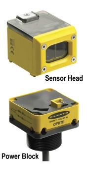
OMNI-BEAM is a modular self-contained sensor made up of a sensor head and a power block. An optional plug-in timing logic module may be added easily. The three modular components, sold separately, plug and bolt together — without interwiring — to create a complete, self-contained photoelectric sensor tailored to a particular application's exact sensing requirements.
