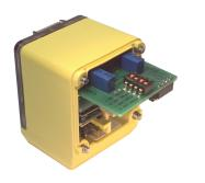
Timing logic may be added at any time, using one of three timing delay and pulse logic modules. Installation is simple and quick; the logic modules simply slide into the sensor head. Program them for timing functions and ranges via four DIP switches; each module includes easily accessible 15-turn clutched potentiometers for accurate timing adjustments.
