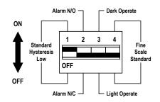
Figure 1. OMNI-BEAM DIP switch location
