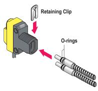
Figure 3. Installing Glass Fibers
