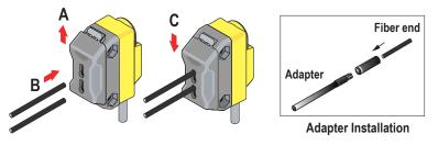
Figure 2. Installing Plastic Fibers
