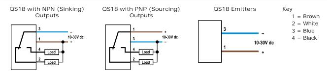
Quick disconnect (QD) wiring diagrams are functionally identical.
