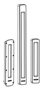
Banner's WLC60 Heavy Duty Lights are engineered to withstand harsh environments, making it the first choice for a machine lighting solution. A conservative mechanical design protects against liquid ingress and state-of-the-art LED technology delivers best of class brightness.
