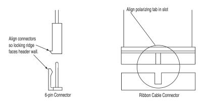
NOTE: If the 6-pin connector is installed backwards, the power light on this module (and possibly the entire assembly) will not light when powered up. Correct this by separating the modules and locating the reversed 6-pin connector.
