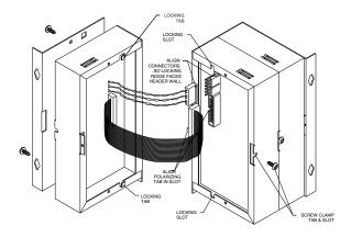
Repeat the procedure for the rest of the modules to be included in the assembly.
