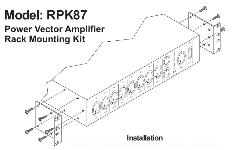
Power Vector amplifiers may be mounted in 19" racks using the RPK87 rack mounting kit. After having attached the rack ears, place the amplifier into the rack and secure it to the rack with appropriate hardware (not included).
