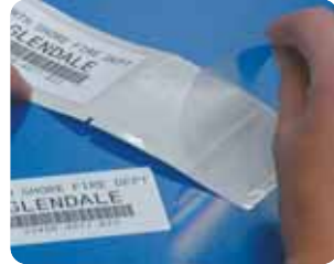
2. Standard label is applied to surface. Laminate is removed from liner.
