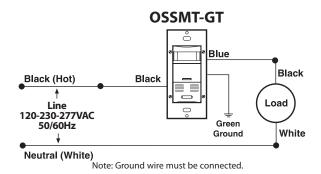
OSSMT-GT Wall Switch Vacancy Sensor Wiring Diagram, Single Location Control
