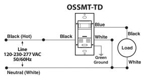
OSSMT-TD Wall Switch Vacancy Sensor Wiring Diagram, Single Location Control
