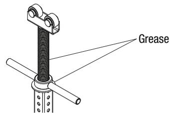
To maximize efficiency and extend the life of the product, apply a thin coat of grease to the threaded shaft and a moderate amount of grease between the thrust washer and underside of the handle. For best results, apply grease before each use.
