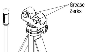
To maximize efficiency and extend the life of the product, re-grease the rollers on the reel stand using the grease zerks found in the center of the roller axles.
