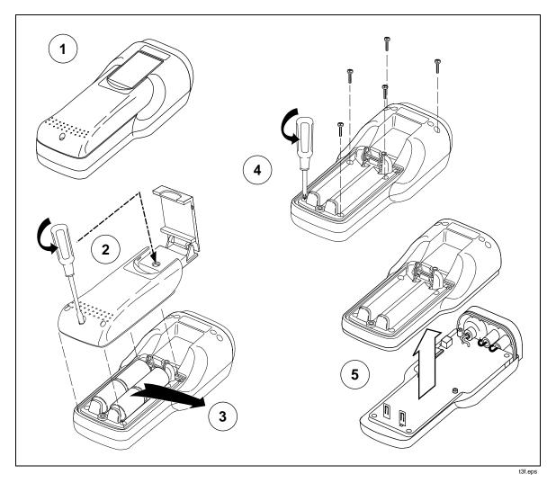
Figure 3-1. Removing the Case Bottom
