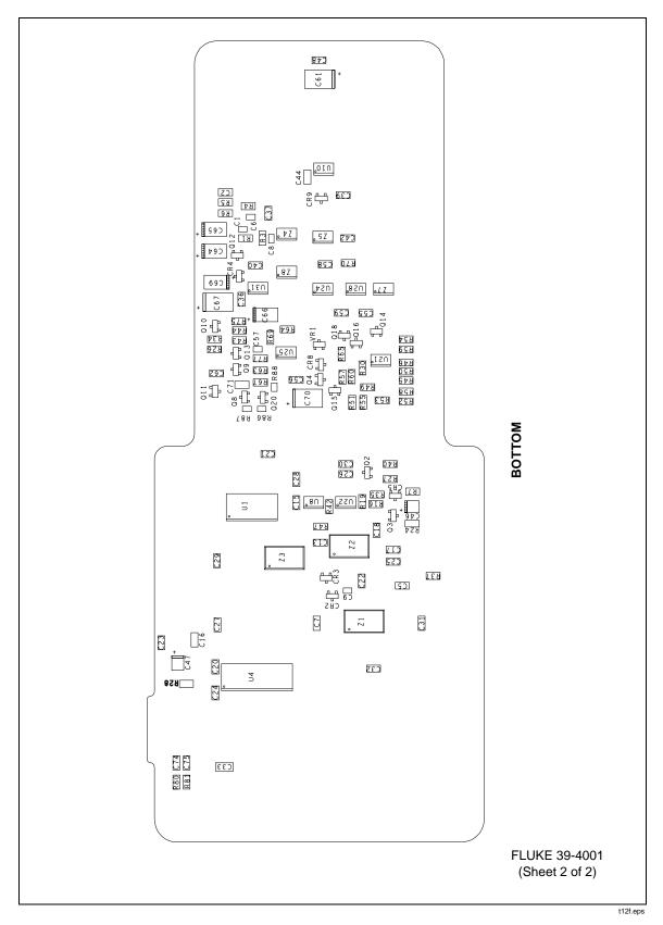
Figure 6-2. Fluke 39 A1 Main PCA (cont)
