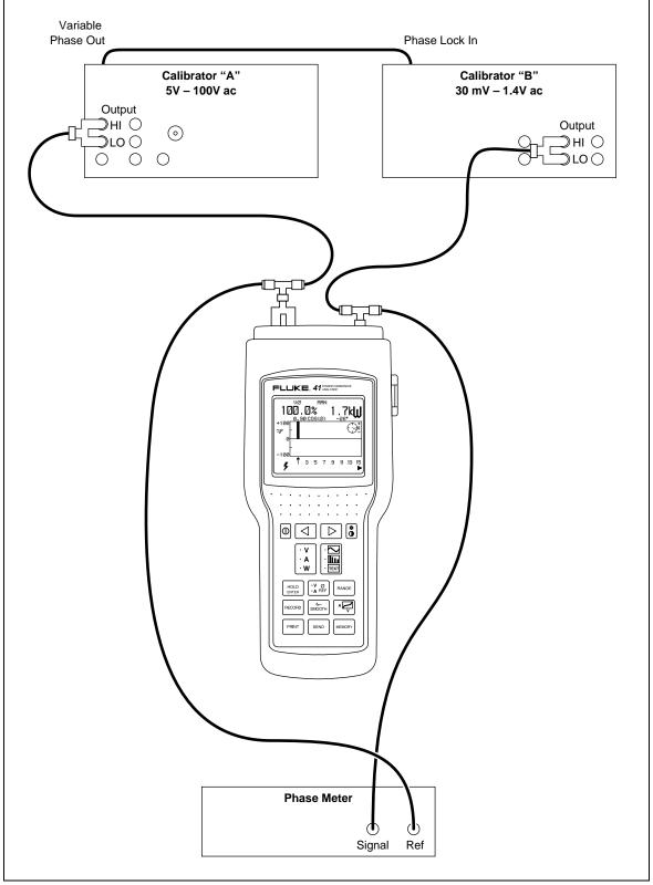
Figure 4-1. Watts Performance Test Configuration
