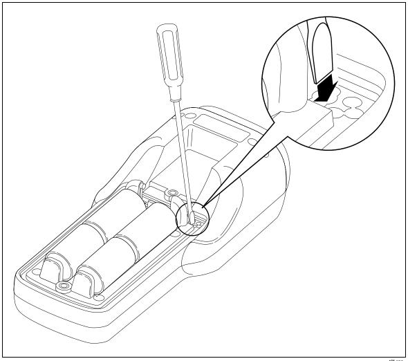
Figure 4-4. Calibration Access Hole
