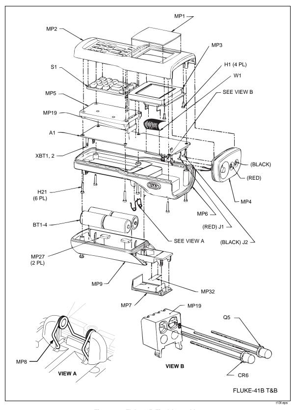
Figure 6-3. Fluke 41B Final Assembly
