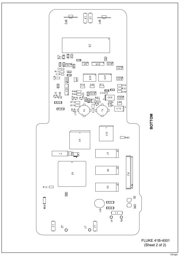
Figure 6-4. Fluke 41B A1 Main PCA (cont)
