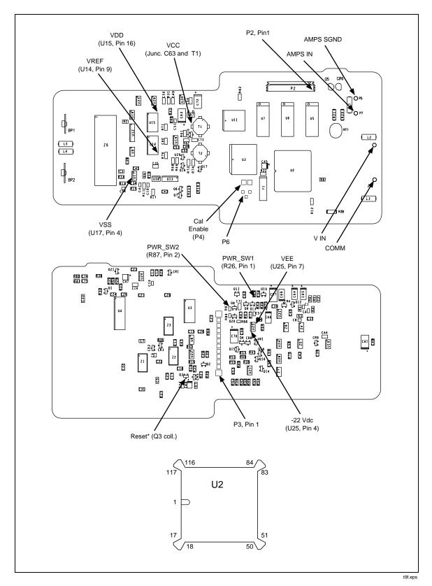
Figure 5-1. Test Point Locator
