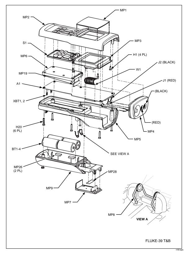
Figure 6-1. Fluke 39 Final Assembly
