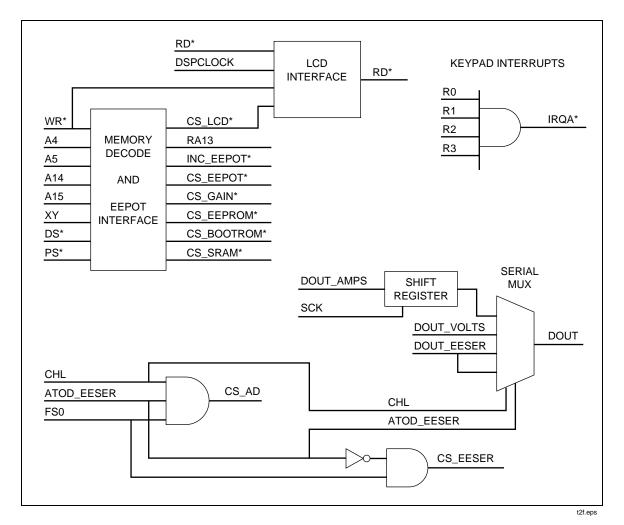
Figure 2-2. PLD Block Diagram
