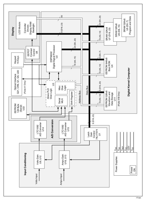
Figure 2-1. Overall Functional Block Diagram
