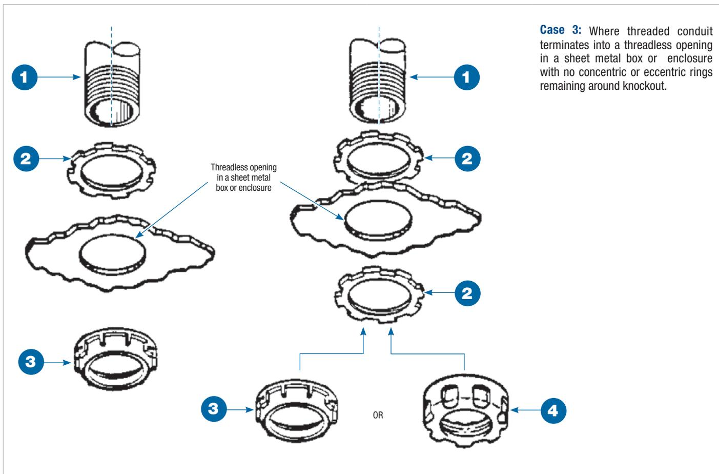
**Case 3:** Where threaded conduit terminates into a threadless opening in a sheet metal box or enclosure with no concentric or eccentric rings remaining around knockout.
