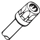
1. Cut conduit end squarely. Remove sharp edges and burrs on inside and outside diameters by reaming or filing.
