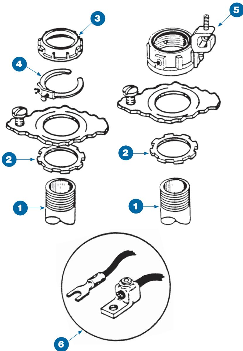
**Case 4:** Where threaded conduit terminates into a threadless opening in a sheet metal box or enclosure with concentric or eccentric rings remaining around knockout.
