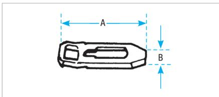
Used with T&B conduit straps to permit space between conduit and mounting surface. Eliminates need for costly offset-bending conduit and possible corrosive moisture traps when conduit is mounted directly to a surface. Hot-dipped galvanized finish, pre-mountable and stackable to eliminate offsetting.
