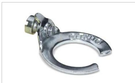
Especially suited for grounding old work, but equally convenient for new, grounding wedges provide grounding without a jumper except in concentric knockouts. When a jumper is required, it fits under a set screw in the grounding wedge.
