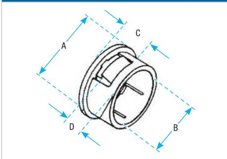
One-piece knockout bushing quickly snaps into outlet box, switch box, or other enclosure left vacant by wiring modifications or maintenance changes. Provides smooth, rounded insulation surface for easy wire pulling. Easily installed by hand, they are available to fit 1/2 in. through 2 in. knockouts. UL Listed 105°C. High impact thermoplastic.
