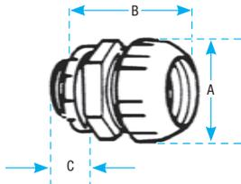
A split steel ring with diagonal serrations grips the conduit and bites into it for positive ground. Makes a permanent connection and eliminates the need for cutting a thread on the conduit. Insulation helps to guarantee continuity of service with protection of the conductor at the critical point — the fitting bushing.
