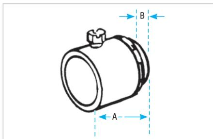
Eliminate conduit threading with these set screw fittings. Captive hex head screws tighten down onto conduit for positive holding strength and ground. The fittings are furnished with insulated throats reducing wire pulling effort by as much as 50%. Approved concrete-tight.
