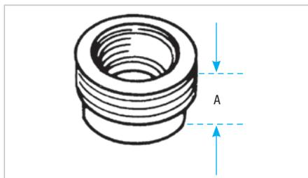
For reducing the threaded opening in conduit bodies or any female threaded fitting. Smooth, built-in bushing completely covers rough ends of conduit. Iron or steel construction. Steel from 600-TB thru 606-TB, also 614 & 615.
