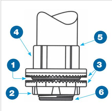
**1. Sealing ring and groove** with innovative profile outperforms standard 'O' ring design. Sealing ring is captive before installation and resists buckling or slipping during installation. The seal groove is designed for optimum compression of the sealing ring. The sealing ring is designed to provide a complete 360° seal, even when the conduit is not perpendicular with the enclosure. (See Figure 1)
