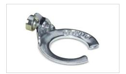
Especially suited for grounding old work, but equally convenient for new, grounding wedges provide grounding without a jumper except in concentric knockouts. When a jumper is required, it fits under a set screw in the grounding wedge.
