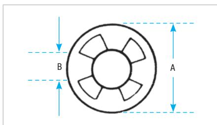
Washers reduce knockout hole in outlet box. Newly designed of galvanized steel. These washers, used in pairs, interlock and form a rib which centers the washers and conduit in the knockout.
