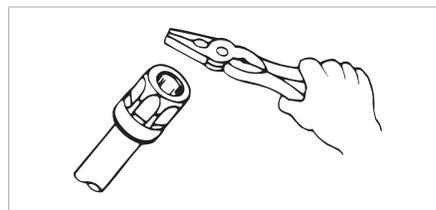
3. Using the flat surface of any standard utility tool such as an electricians pliers (or a hammer with a block of wood, for the larger sizes), strike the bushing on its top surface using a Series of light blows until the end of the conduit rests against the bushing throat and conduit stop.
