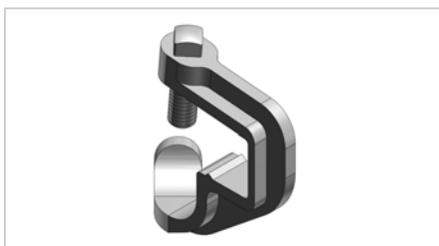
These supports will fit any flange, tapered or straight up to 5/8 in. thick. The broad hook holds the conduit at any desired angle. Holds standard rigid conduit, EMT, or I.M.C. Malleable iron.
