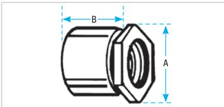
With an Erickson® coupling, a conduit run may be completed when neither conduit can be turned. A conduit run may also be broken without taking down the whole run. Conduit joined with Erickson® Couplings is rigid and in line and vibration will not loosen the connections.
