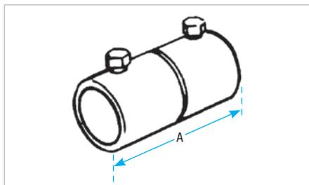
Eliminate the need for threading conduit ends when joining rigid conduit with these set screw couplings. Captive hex head screws provide positive holding strength and ground continuity. Approved concrete-tight.
