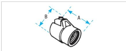
A one-piece fitting that couples armoured cable or flexible conduit to threaded rigid conduit. Tite-Bite® wedge holds conduit securely with a double grip. With a Chase® nipple, this fitting will connect flexible conduit to outlet boxes, allowing more wiring space in the box than the usual fitting. Malleable iron.
