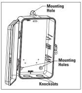
Position at eye level if possible, providing space to the left of the enclosure for the cover to swing open fully, as shown.
