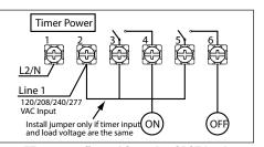
ET8215 configured for pulse SPST load with jumper set to PUL
