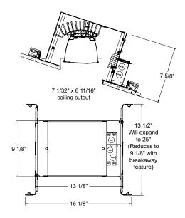
**Junction Box** Pre-wired junction box provided with (6) 1/2" and (1) <sup>3</sup>/<sub>4</sub>" knockouts, (4) non-metallic sheathed cable connectors and ground wire, UL and cUL listed for through-branch wiring, maximum 8 #12 branch circuit conductors • Junction box provided with removable access plates • Knockouts equipped with pryout slots • Push-in electrical connectors supplied as standard for fast, secure installation.
