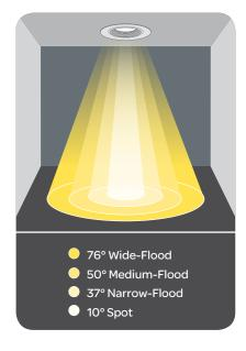
Juno Generation 3, 5" and 6", IC-Rated, 600 & 900 Lumen LED Downlights are available in four optics. Wide-flood beam pattern is standard; medium-flood, narrow-flood and spot are also available. Reflector styles can be changed easily via the convenient twist and lock accessory feature.
