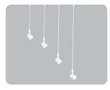
Line voltage extension wands suspend all Juno line voltage track lights (with square Super Adapter only) from all Juno Trac. May also be used with Monopoint connections. Can be used on all 120V track. Constructed of 1/2" rigid tubular steel and Lexan® plastic.
