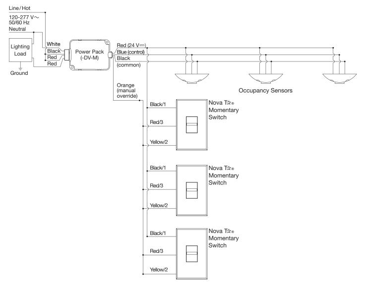
**Note:** A maximum of 3 devices can be used with PP-DV-M/UPP-DV-M. Each PP-SH/UPP-SH counts as 1 device, each occupancy sensor counts as 1 device. Nova T☆<sub>®</sub> momentary switches are not included in this count.
