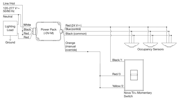
**Note:** A maximum of 3 devices can be used with PP-DV-M/UPP-DV-M. Each PP-SH/UPP-SH counts as 1 device, each occupancy sensor counts as 1 device. Nova T☆<sub>®</sub> momentary switches are not included in this count.
