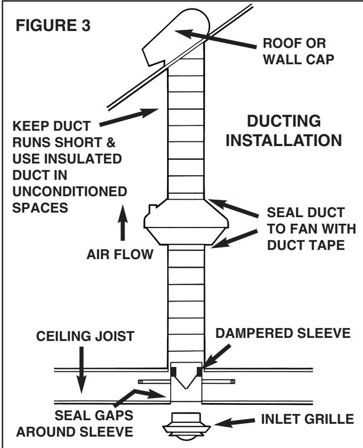
The ducting from this fan to the outside of the building has a strong effect on the air flow, noise and energy use of the fan. Use the shortest, straightest duct routing possible for best performance, and avoid installing the fan with smaller ducts than recommended. Insulation around the ducts can reduce energy loss and inhibit mold growth. Fans installed with existing ducts may not achieve their rated airflow.
