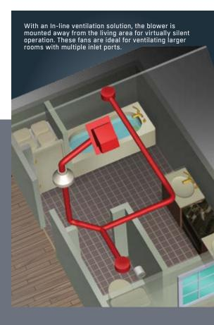
**Remote Mounted In-Line Ventilation Fans** are quiet and efficient residential solutions. The concept is simple: mount a high-performance ventilator in an out-of-theway spot and you get the power with virtually no sound.
