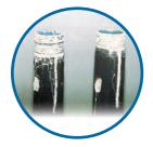
Examples of Hot-Dip Galvanized Threads after 42-day salt-fog test
