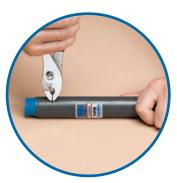
In Step 3, the tab is pulled perpendicular to the conduit with a pair of pliers. The plastic tab will tear off rather than having any peeling effect or the coating separating from the substrate.
