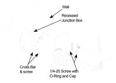
FIG 2 RECESSED JUNCTION BOX INSTALLATION
