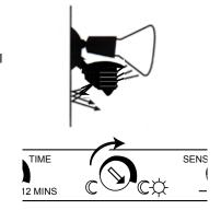
2. Check if "R" lamps, non-reflector "A" lamps or self-ballasted PL lamps are being used in non-enclosed lampholder. If so, switch to reflector PAR floodlight lamps so the sensor is not affected by stray light. If using PAR floodlights, consider using lower wattage, energy saving lamps.
