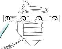
The best location is where the sensor can "see" all paths of movement. The sensor may be wall or soffit mounted.
