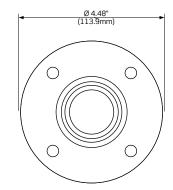
Mounting Pattern Common to Both Male & Female Configurations
