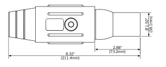
Ball Nose In-line Latching Female Plugs S-Series
