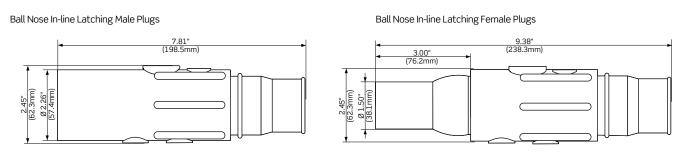
Ball Nose In-line Latching Male Plugs S-Series
