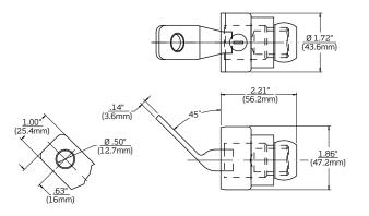
18F22 Female Terminal Connector - Bus Bar Mount, Offset
