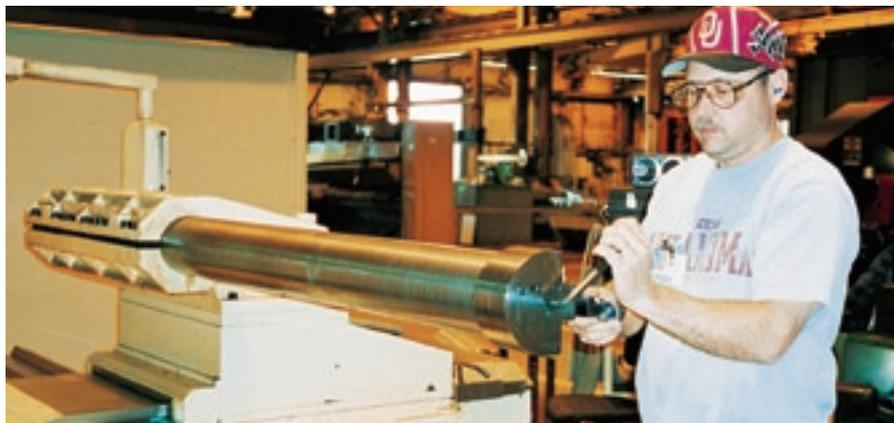
A long tuned boring bar on a flat-bed lathe.
