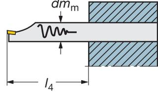
**Tuned damped bar**
