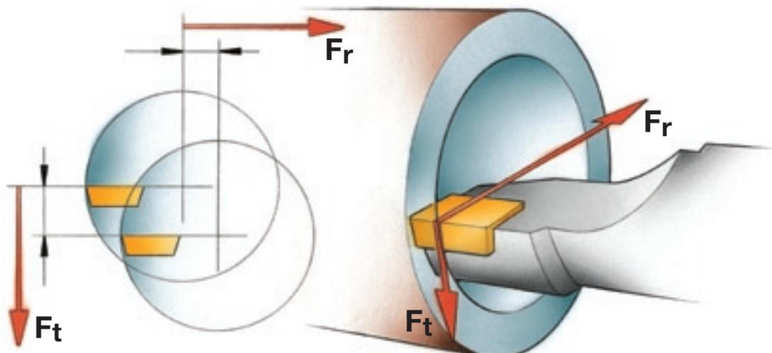
Radial and tangential cutting forces deflect the boring bar during machining, often necessitating cutting edge compensation and tool damping.
