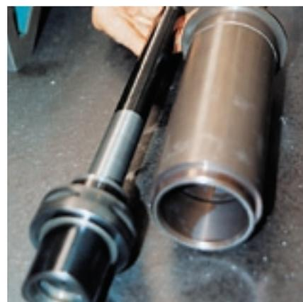
Tool clamping at the front end and back end are important performance factors for machining with long boring bars.
