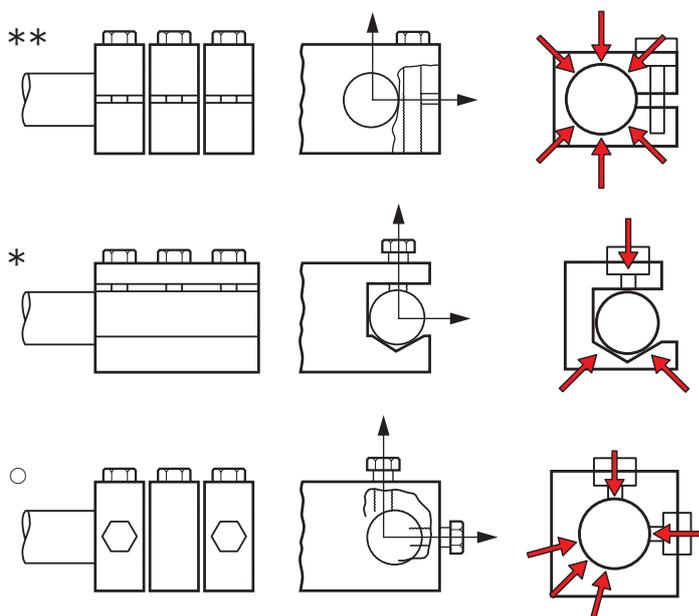
The way a boring bar is clamped is decisive as regards performance and results (\*\*\*) = best, \*\* = acceptable, \* = unacceptable, ○ = not recommended.)
