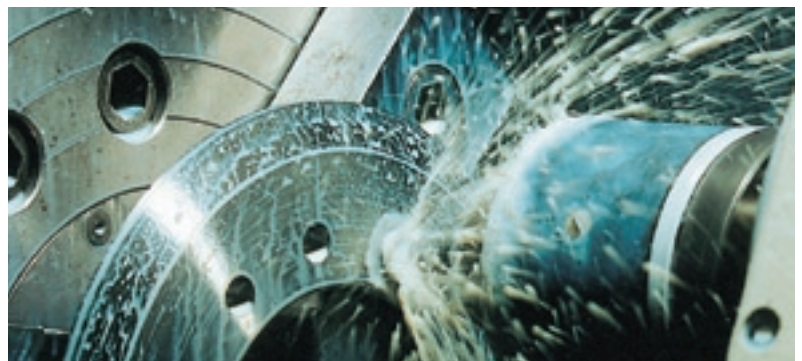
Suitable cutting fluid supply is critical in drilling.
