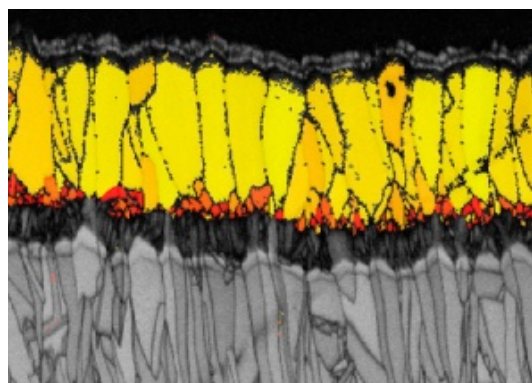
With Inveio, every crystal in the alumina coating is lined up in the same direction, towards the top surface.
