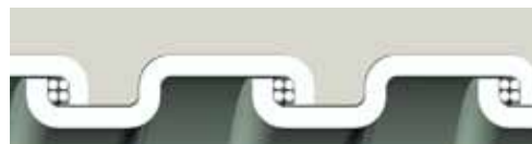
Square-Locked Design with cord packing 3/8" through 1-1/4"
