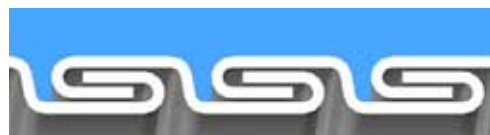
Interlocked Design 1-1/2" through 3" with no bonding wire
