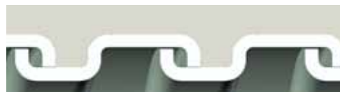
Square-Locked Design 3/8" through 2"
