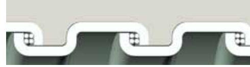
Square-Locked Design with cord packing 3/8" through 1-1/4"
