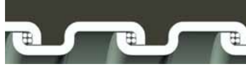
Square-Locked Design with cord packing 3/8" through 1-1/4"
