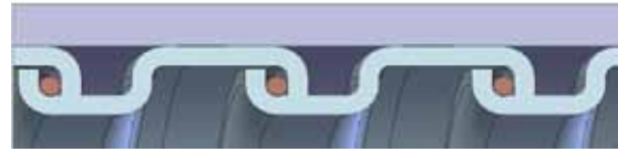
Square-Locked Design with integral bonding wire 1/2" through 1"
