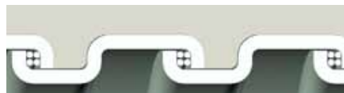
Square-Locked Design with cord packing 5/16" through 1-1/4"
