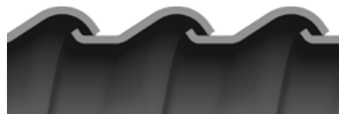
Angle-Lock Design 3/8" through 4"
