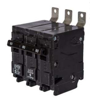
Siemens Low Voltage Molded Case Circuit Breakers Panelboard Mounting 240V Circuit Breakers - Type BL, 3-Pole, 240VAC are Circuit Protection Molded Case Circuit Breakers. Type: HBL Special Features: Shunt Trip 120V Application: Electrical Distribution Standard: UL 489 Voltage Rating: 120/240V Amperage Rating: 60A Trip Range: Thermal Magnetic Interrupt Rating: 65 AIC Number Of Poles: 3P
