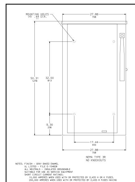
CLASS R REJECTION KITS INSTALLED OR CLASS J FUSES.
