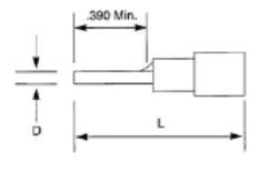
Provides an easy and effective way to terminate stranded wire into European/metric-style terminal
