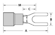
Inner bronze insulation grip sleeve lengthens flex radius of conductor and eliminates conductor creep. Nylon jacket is color-coded.
