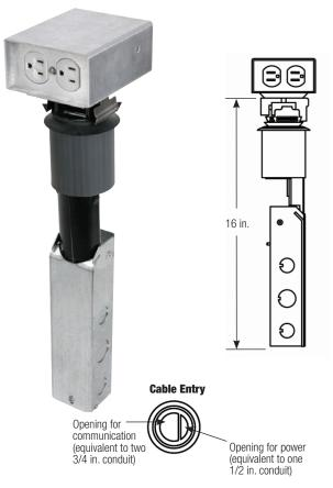
By mounting all outlets above-floor level and at a  $90^{\circ}$  angle to the floor, the FPT Pedestal Series protects power receptacles and communications devices from dirt and debris. An overhanging housing provides additional protection for the outlets.
