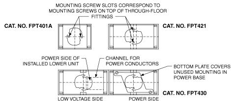
Cat. No. FPT430 is offset with respect to through-floor fitting which mounts under low voltage base with power side of through-floor fitting closest to power base.
