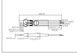
In order to protect the surrounding environment, this surge protection device must be enclosed in a luminaire that can contain flames and sparks, which may occur in case of malfunction, such as overvoltage power connection (ex: 600V).
