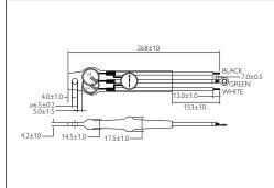
In order to protect the surrounding environment, this surge protection device must be enclosed in a luminaire that can contain flames and sparks, which may occur in case of malfunction, such as overvoltage power connection (ex: 600V).
